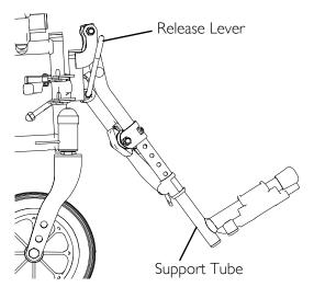
FIGURE 4.5 Raising/Lowering Elevating Legrest Assembly
